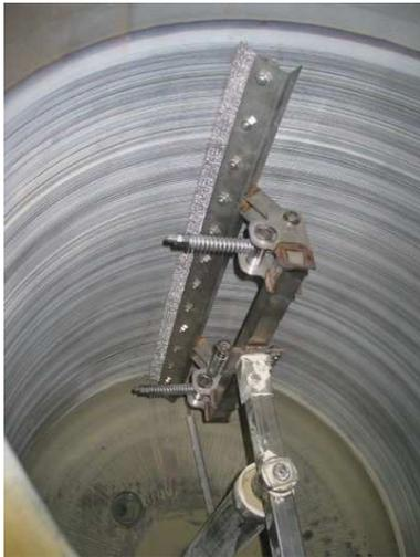
The HP-R series use a heat pump system and has external heating coils and features an internal boiler scraper to avoid the build-up of encrusting solids on the boiler surface.
